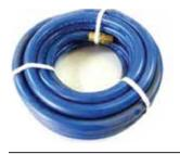
A lightweight, economical general purpose hose for carrying air, water, and many spray solutions. Pliovic is suitable for a wide range of industrial, construction and agricultural hand sprayers, and many multipurpose applications. Rated to temperatures of -10°F to 158°F (-23°C to 70°C). Nonconductive, minimum electrical resistance greater than one (1) megohm per inch of hose length at 1000 Volts DC. Available in Pliovic GS construction or a thick cover, Pliovic Plus construction.
