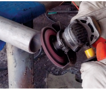
Grinding and beveling stainless steel tubing with a Saber Tooth abrasive flap disc.
