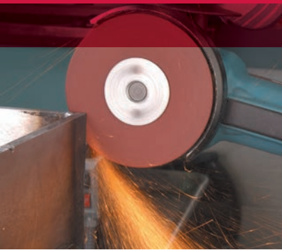
Blending welds on the corner of a steel furniture frame.
