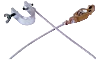
Part# 272031 - .53 lbs All Purpose Bond Wire: For bonding drums to each other, to containers being filled, and to racks. Three-foot-long heavy duty wire rope with "C" clamp on one end and alligator clip on the other.
