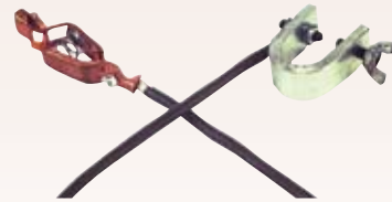
Part# 272032 - .64 lbs Deluxe Ground Wire: For connection between drum and true ground. Three-foot-long heavy duty insulated wire rope with "C" clamp on one end and alligator clip on the other.
